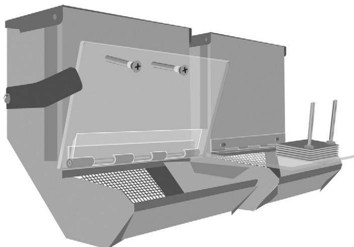
**Fig. 1.** Feeders as mounted on the center rear wall of each subject's cage. The feeder on the left is shown in the free position (lid locked open), while the feeder on the right is in the closed position, with several 33 g weights positioned on two machine screws to increase the cost of access to pellets or wooden cubes.
